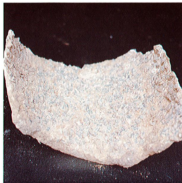
Remainder of bottom third of 225 mm O-G jointed concrete pipe from a sewer downstream of a pumping main discharge which had failed after less than 10 years service. The aggregate exposed after the cement had been attacked by sulphuric acid oxidised from atmospheric hydrogen sulphide in the presence of moisture is clearly visible.
